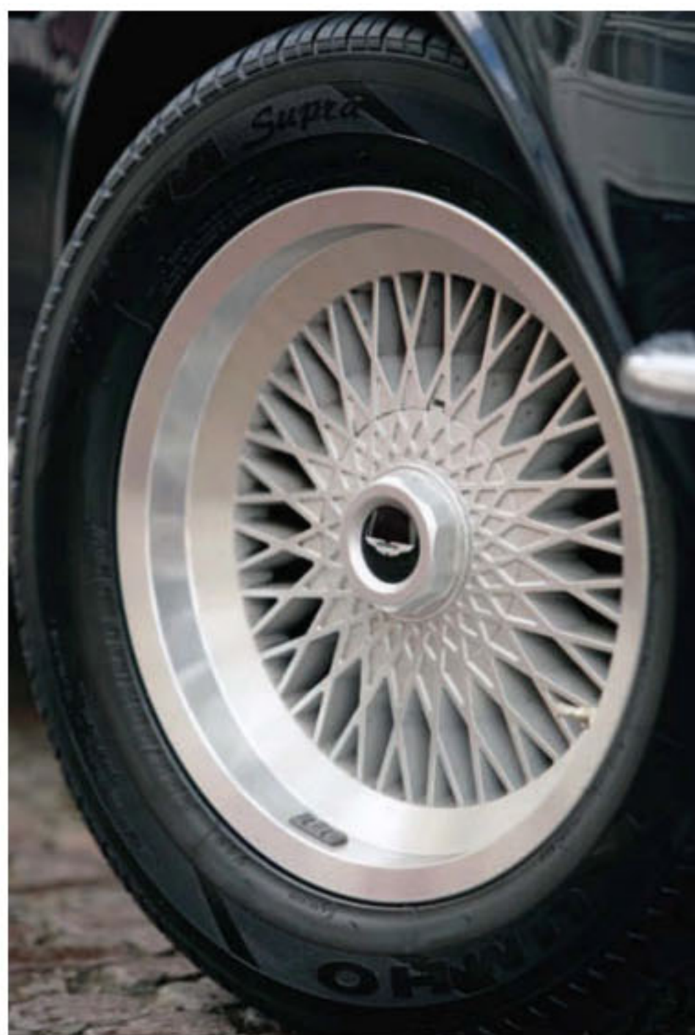
Above: cabin is superbly appointed but not to all tastes. Left: 16in cross-spokes shout 1980s, but car handles well on its 255/50 Kumho tyres
