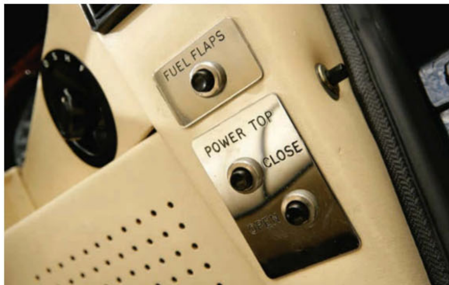
Clockwise, from above: Mick Durrant built this quad-cam V8; Smiths motor rapidly raises hood – fuel flaps are also electric; build plaque an Aston constant
