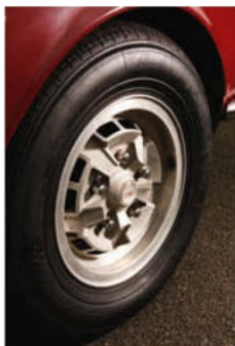
Clockwise, from above: DBS was last car to carry traditional chrome face before smooth, twin-lamp nose of AM V8; Marek's V8 with troublesome fuel injection; bespoke GKN alloys, with vents to cool the overworked brakes
