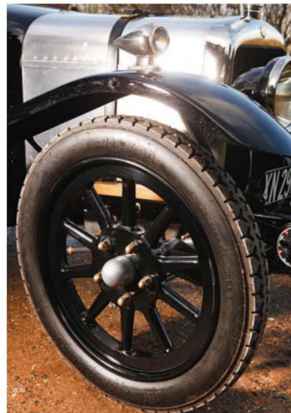
Clockwise: single-carb sidevalve 'four' musters 40bhp, but A3 struggles up hills; charming chassis plate; 'Sankey' wheels were recreated in aluminium
