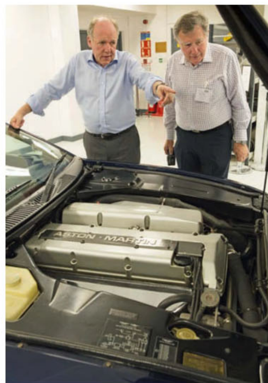
Clockwise, from top: design team that readied the car for launch; Callum points out that the ‘six’ was lowered rather than altering bonnet line; fully engineered prototypes – sunroof of early cars was dropped as a standard item; Geneva debut, ‘93; Bloxham works, where the XJ220 had also been built
