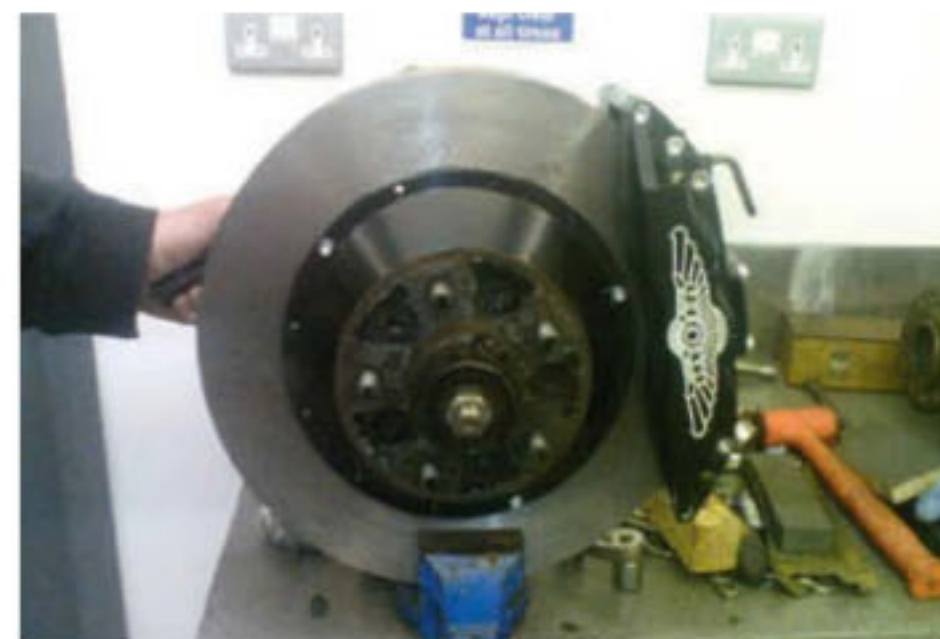
Taylor developed bespoke brakes with six-pot calipers
